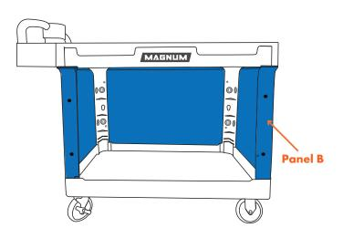
Attach Panel A to Panel B using four 8mm Hex Bolts with Flat Washers and 8mm Flange Nuts with Split Washers (Every other hole from the top as illustrated below). Make sure all seven holes are aligned.
